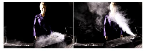
Figure 2. Smoke visualizations of the dispersion of the patient exhaled air. The case with local downward supply is shown on left and with overhead mixing on right. The diffusers were placed in the ceiling above the patient in both cases.
