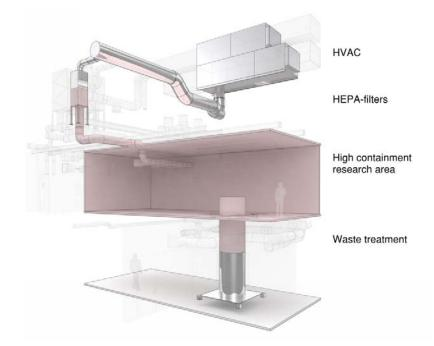
Figure 1. High containment facility geometry. The principle of the containment barrier, as illustrated by M. Jepsen, Henning Larsen Architects<sup>6</sup>.
