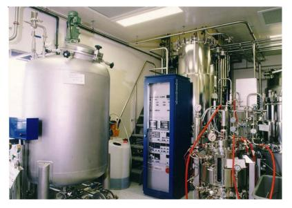
Figure 3: Un-cleanable bioreactor by congestion and poor design
