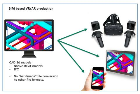
Figure 2. VR/AR models are created from a single source
